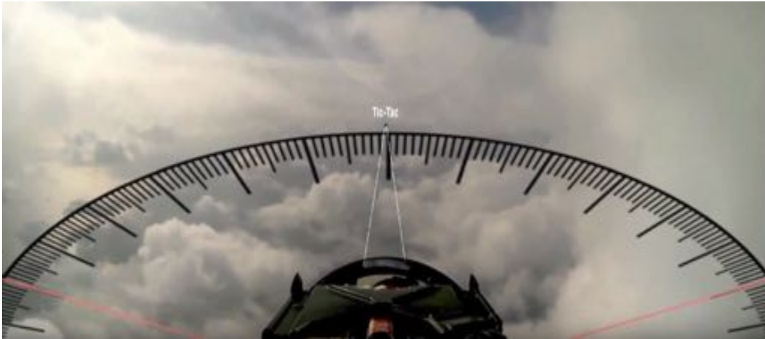
Figure 1: shows the small angular area aperture of 1.5 deg of the ATFLIR
